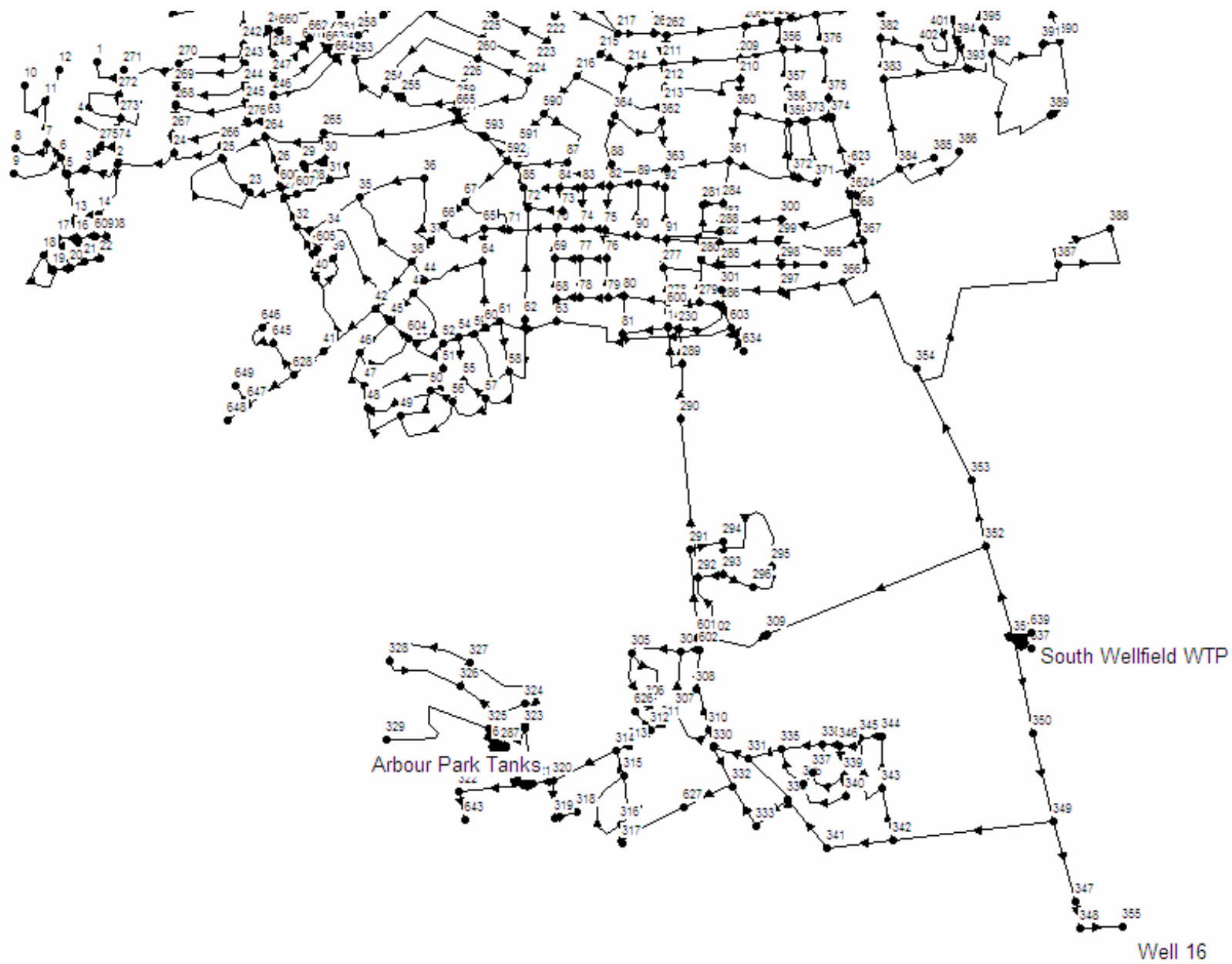
Figure 7. Southern service areas in the City of Newark water distribution model.
