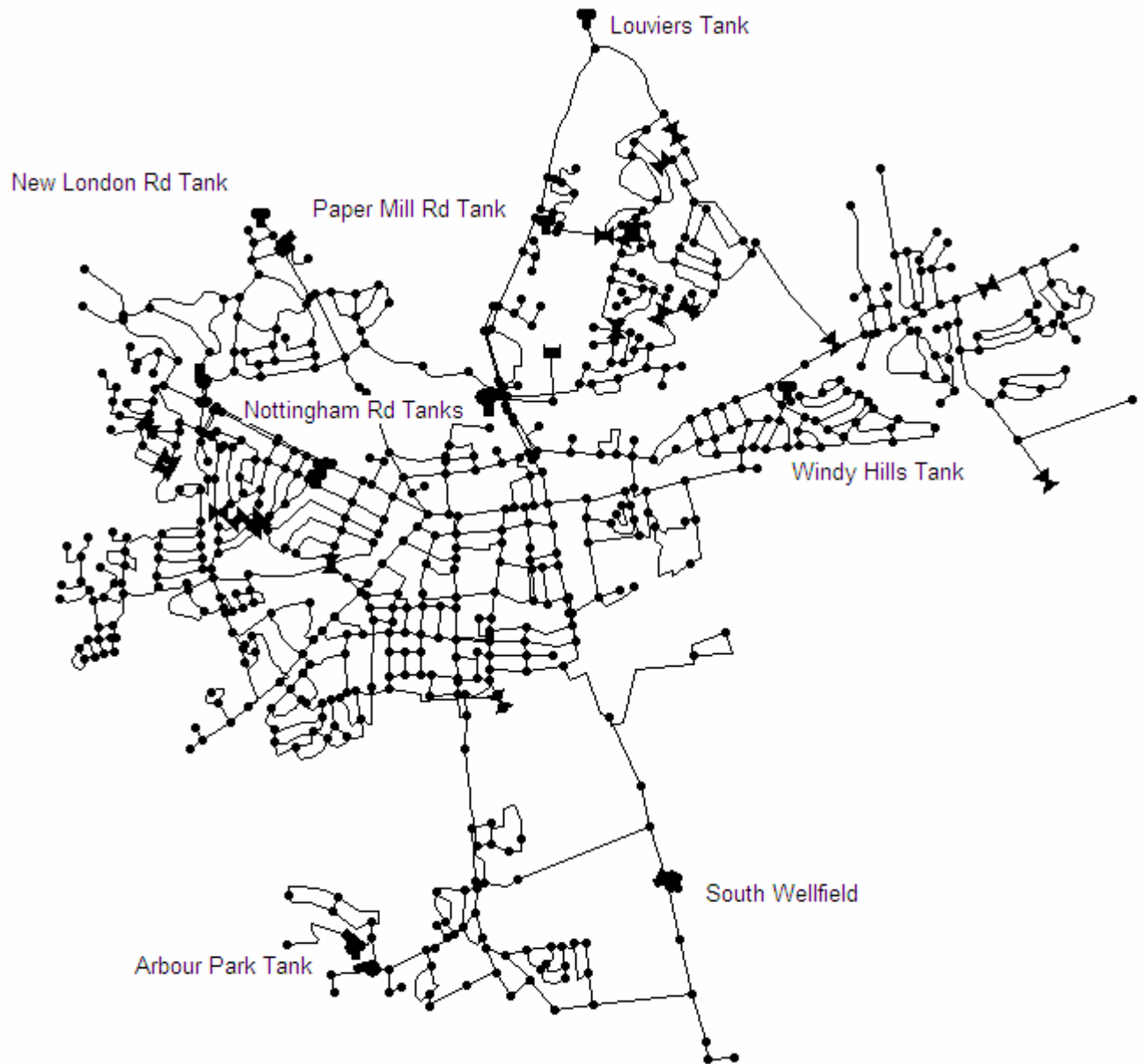
Figure 5. City of Newark EPANET 2 water distribution model with wells and tanks.
